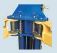
The supporting arms are automatically locked in position during the lifting operation. Once the lift has been completely lowered, this interlock is automatically released. The very narrow spacing between the locking positions and a manual unlocking function enhance the ease of use.
